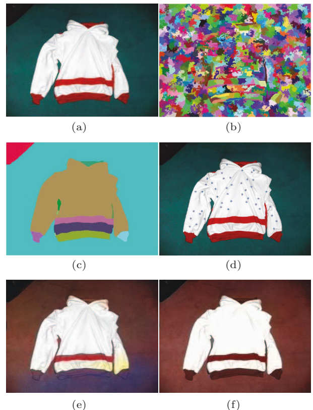
Fig.5. One example of color consistency evaluation. (a) Ground-truth color image. (b) Superpixels generated by graph-based segmentation on pixelwise color vectors \mathbf{f}_c = (k \times l, a, b)^T (shown in random colors). (c) Hierarchical image segmentation results (shown in random colors). (d) Selected point group for consistency evaluation (shown in blue asterisks). (e) State-of-the-art colorization result by [19], \hat{\sigma}^r = 7.91 . (f) Our result, \hat{\sigma}^r = 1.43 .
